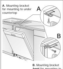
*bent* for mounting to side of cabinets
